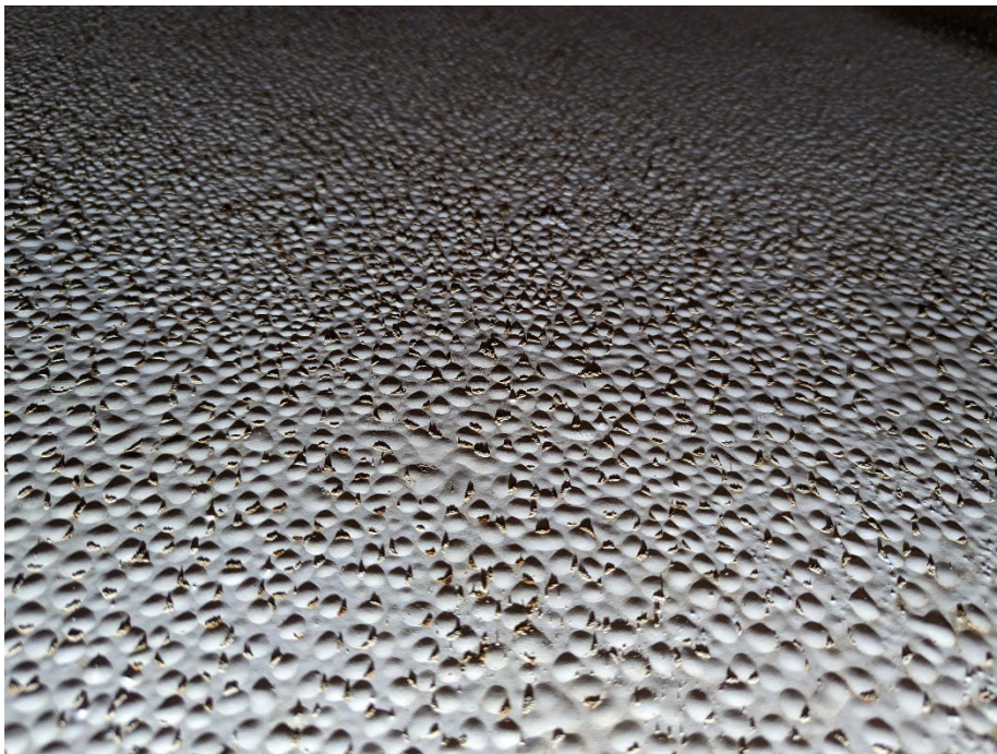
Photo 5 – Typical Blisters on Bottom Plates
